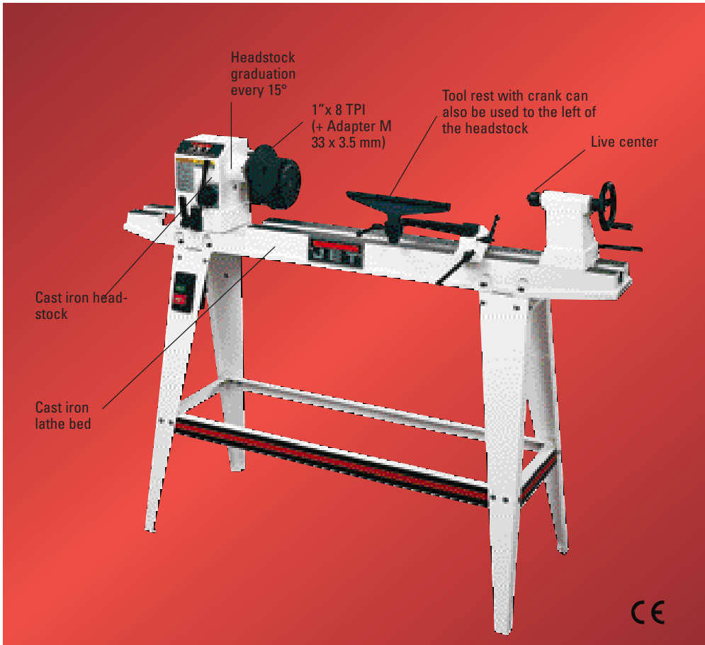
Pivoting headstock quickly turns and locks to facilitate outboard turning and to provide better vision during internal machining
