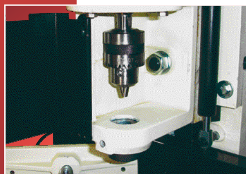
Large hinged chuck door allows easy access to lock the bit in place
