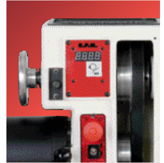
Digital speed display for quick reading of speed
