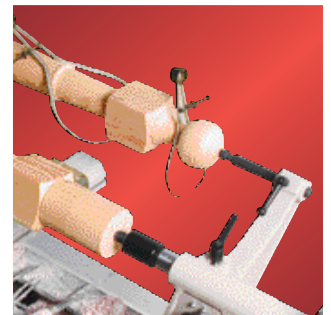
Set of dead centers which hold a spindle for visual comparison
