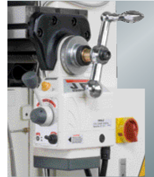
Automatic x-feed with limit switches and quick motion button
