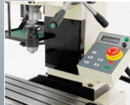
Control panel with digital display for spindle speed
