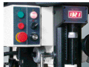
Variable speed control via frequency converter with digital display and right/left-handed rotation; standard with JMD-18VS
