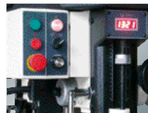
Variable speed control via frequency converter with digital display and right/left-handed rotation; standard with JMD-18VS
