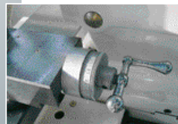
Adjustable graduated collars and chrome-plated hand wheels
