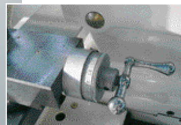
Adjustable graduated collars and chrome-plated hand wheels
